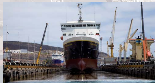
Lifting platform 175 mts long 30 mts wide, up to 10,000 tons net lifting capacity (approx. 36,000 DWT)
